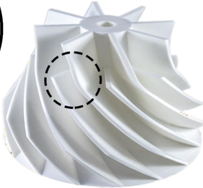
Close up a printed object with PLA-X 3 (Printed on an Ultimaker 2+, 0.19 layer height, 242c)
